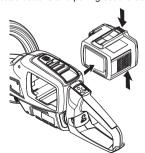
IMPORTANT! Always remove the battery to prevent the machine being started by accident.
